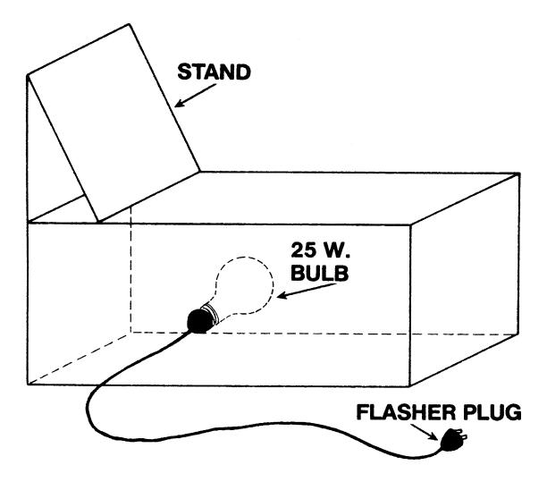
In order to make one of these miraculous instruments you will need a box, an old shoe box will do; a twenty five watt light bulb; a light socket with wire and plug attached (available at any hardware store) and a flasher plug (also available in any hardware store with the exception of those in Queensland, Australia and don't ask me why) and a sheet of wax paper.
